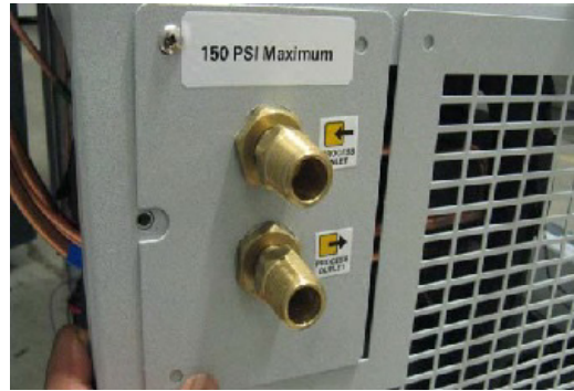
Figure 4. Fittings installed on freezer
