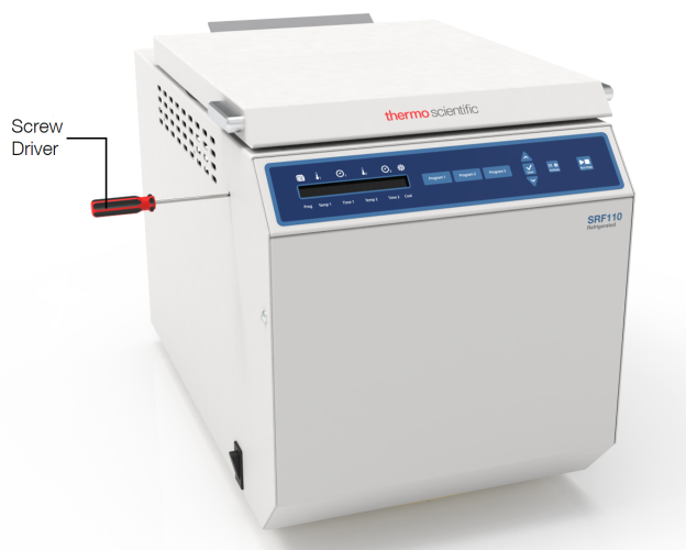
Figure 3. Opening chamber cover in emergency
