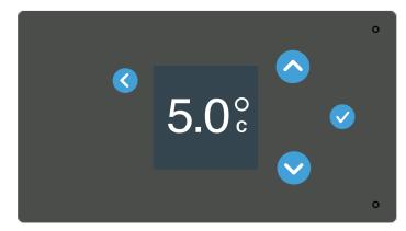
When the unit is first plugged in and powered, the temperature range alarms are not enabled until the unit reaches its preset temperature range + an offset of 3°C. If the set point temperature is 5°C, then the alarms are enabled when the unit reaches 8°C.
