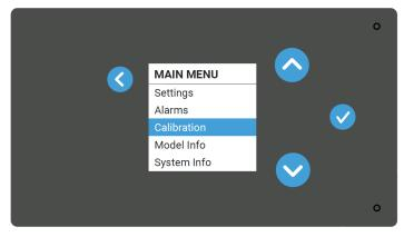
Example: Refrigerator air temperature displays as 3.5°C. Calibrated reference thermometer reads 3.6°C. Based on this information the refrigerator is reading 0.1 degree below the reference temperature. By raising the CALIBRATION to +0.1°C the refrigerator will now display 3.6°C.
