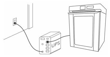
The TSG refrigerator is compatible for use with a UPS battery backup. The primary role of any UPS is to provide short-term power when the input power source fails. If you use a UPS backup, be sure to follow the directions and precautions accompanying that device.
