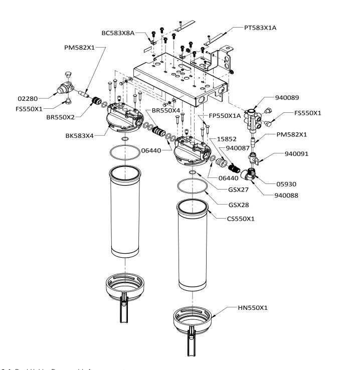
Figure 8-1. Dual Holder B-pure with Aquapro meter
