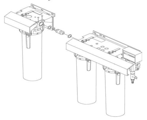
Figure 6-1. Three Holder System (3 Water Treatment Cartridges)
