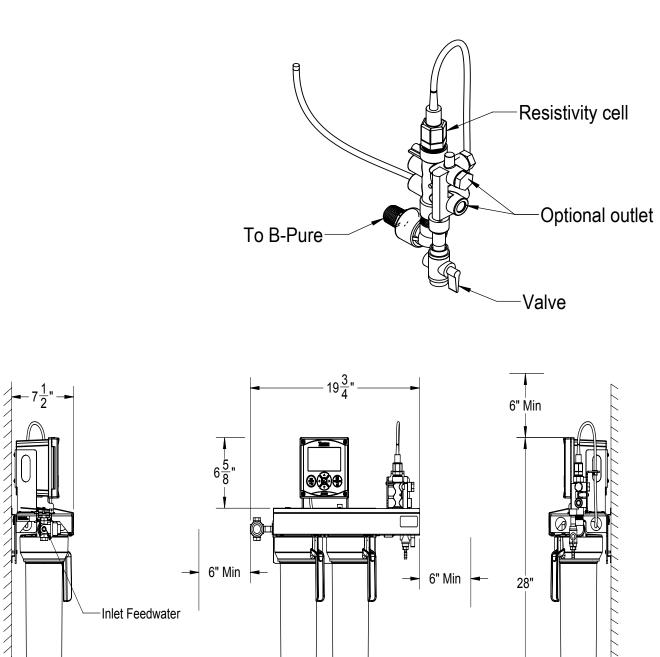
Figure 3-1. B-Pure wall mounted roughing drawing
