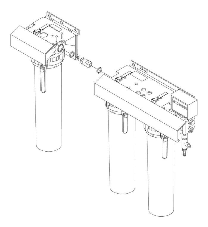
Figure 8-2. Three Holder B-pure (Three Water treatment Cartridges)
