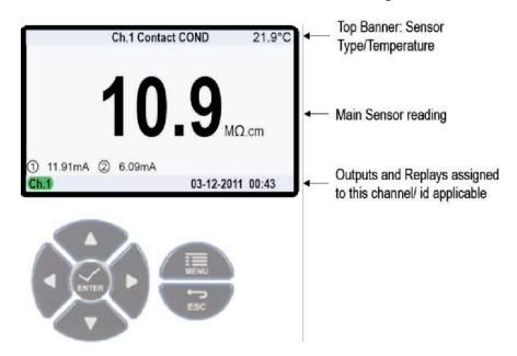
The top line banner displays a User Entered Channel "NAME" to the left, the channel and measurement type in the center and the temperature on the right. By default the "NAME" is blank.
