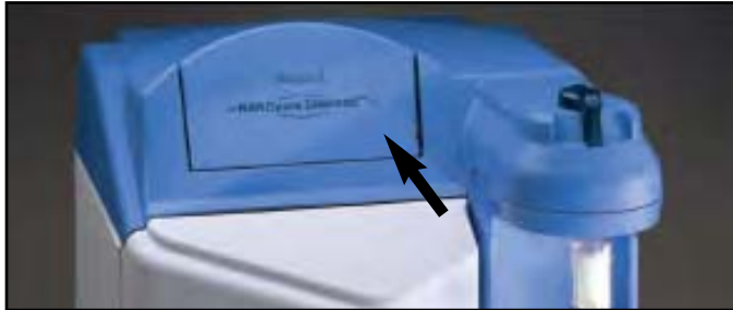
Figure 3-24. Blank Control Panel
