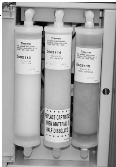
Figure 3-8. Cartridge Installation:(left to right) prefilter, MPS, carbon
