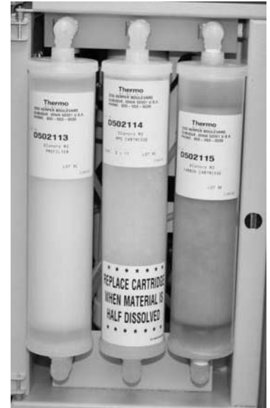
Figure 5-1. Cartridge Installation:(left to right) prefilter, MPS, and carbon
