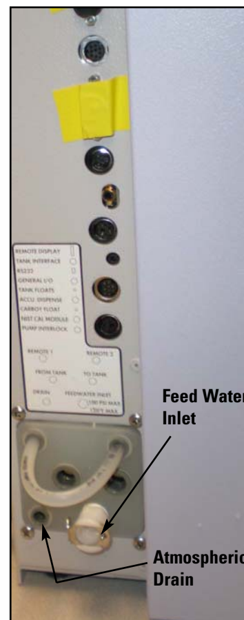
Figure 3-13. Feed Water Inlet and Atmospheric Drain
