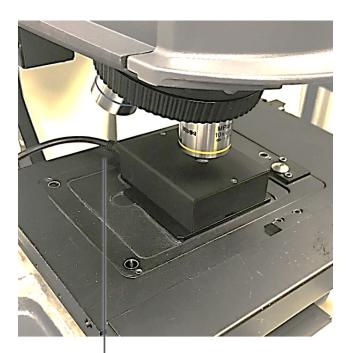
Position the tool so that the cable extends toward the microscope
