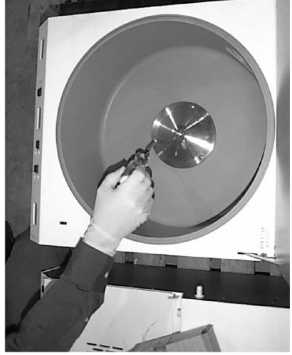
PHOTO LOOKING DOWN INTO SPEEDVAC® CHAMBER AT SUMAX SPD UPPER MAGNETIC ASSEMBLY
