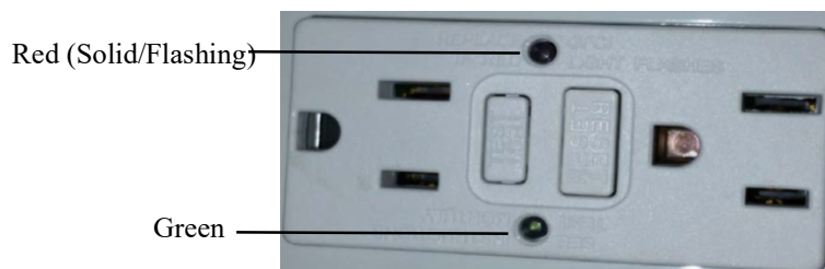
Figure 3. NEMA 5-15 Receptacle Lights
