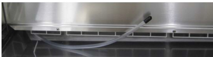
Figure 2. Test ports Herasafe 2030i
