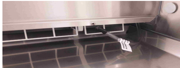
Figure 15. Test ports Herasafe 2030i
