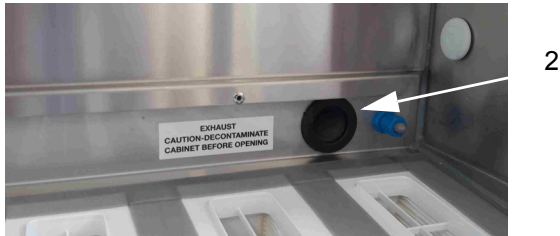
Figure 17. Testing Exhaust Filter
