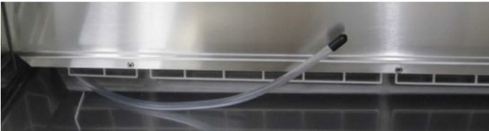
Figure 6. Test ports Herasafe 2030i
