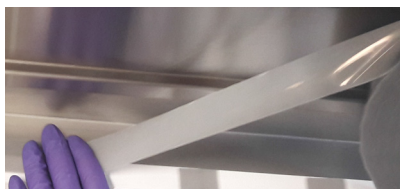
Figure 42. Apply upper sealing
