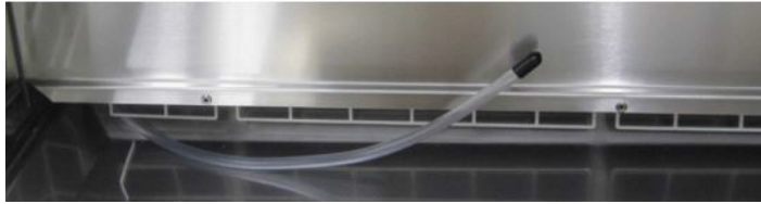
Figure 10. Test ports Herasafe 2030i
