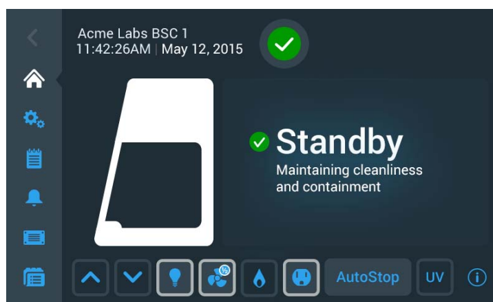
Figure 32 Main Screen - Unit in Standby
