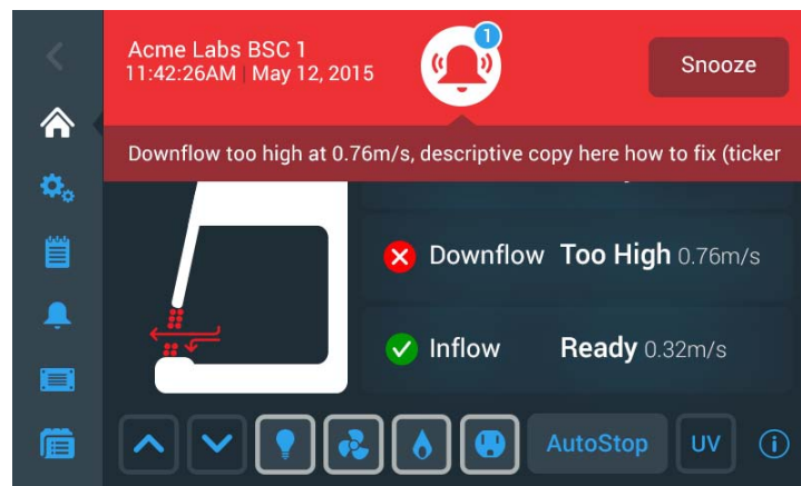
Figure 52 Alarming Screen for Downflow Too High Alarm
