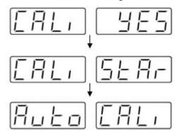
Step 4: Terminate configuration mode as described in Configuration Mode. To cancel the auto-tuning during the process, turn off the main power switch. If cancelled, the Optimal Mode will be selected automatically with an alarm.
