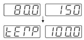
Step 2 : Select the desired temperature by turning and press the Heater Knob.
