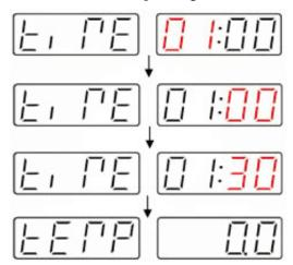
Step 3: Now, the unit will display the set temperature for verification as shown below. Turn the Stirrer Knob to select the desired value and then press it for confirmation. The following display will appear momentarily. [If you change the set temperature]
