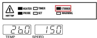
During STIRRER function operating, the stirrer value will be showed on display window. When you push the stirrer knob, you can check current stirrer operating value.
