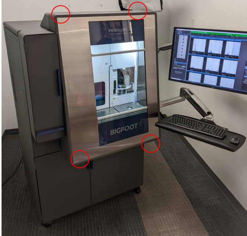
Figure 2: Location of four quarter turn fasteners to remove top front cosmetic cover.
