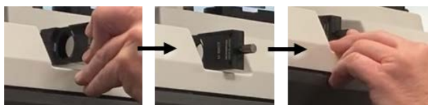
Figure 3-2: Insert Wollaston prism into base slot
