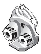
The accessory has two wheels: wheel A is closer to the source. Each wheel can be moved to one of four positions. Both wheel A and wheel B have an open position for collecting spectra without a filter in the beam path. Positions 1, 2 and 3 are available for filters that you provide. Each position accepts one 1 mm thick or one 4 mm thick filter that is 1-inch in diameter. Spacers are provided to secure 1-mm filters in position.
