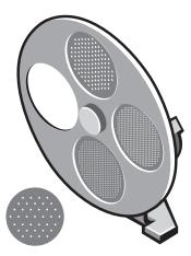
The wheel can be moved to any of four positions: an open position (for collecting spectra without a screen in the beam path) and 3 screen positions. As shipped from the factory, the screen positions are populated with 30%, 10%, and 3% screens. The Screen Wheel parameters in Experiment Setup to describe the percentage of light transmitted by each screen installed in the wheel. Simply select one to move the screen into the beam path.
