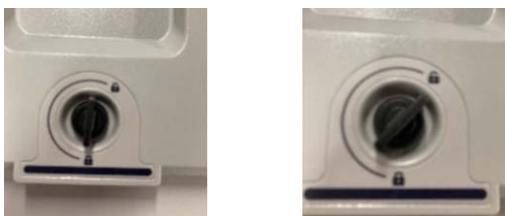
Figure 3-9: Latch: locked and unlocked positions
