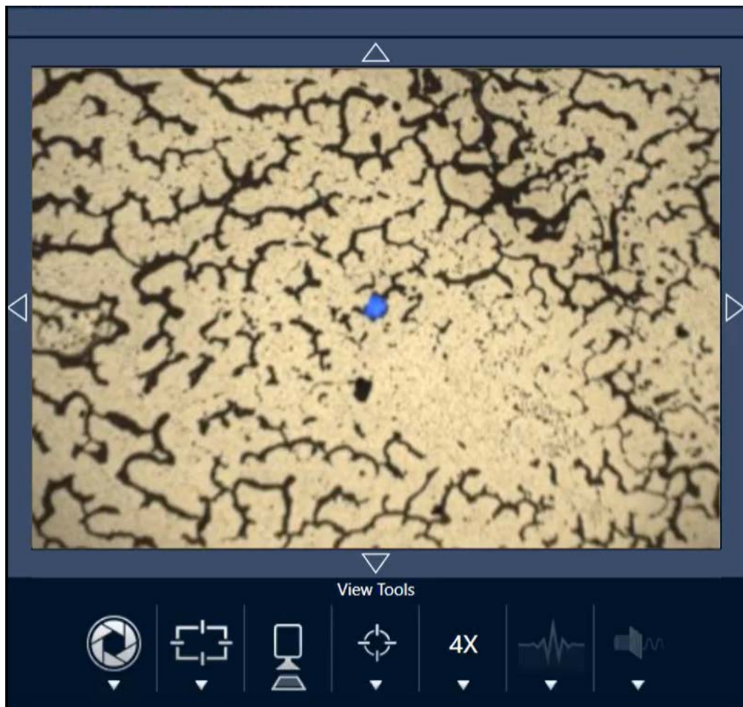
Figure 3-2: Centered sample (dyed fluorescent polystyrene beads) using 4x objective and blue excitation. One bead is seen fluorescing.
