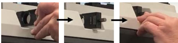
Figure 3-2: Insert Wollaston prism into base slot
