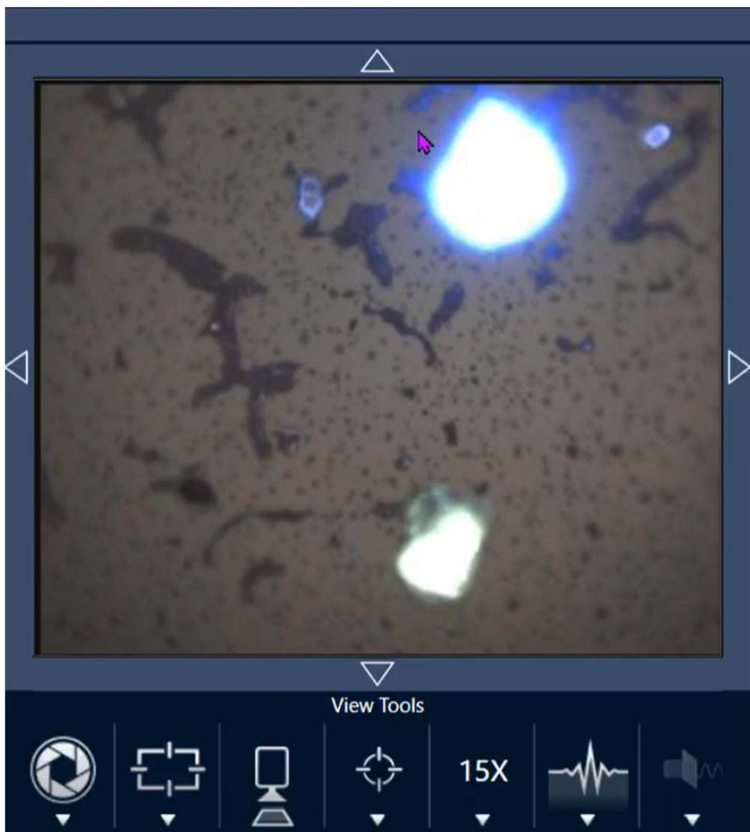
Figure 3-4: Centered sample (dyed polystyrene beads) using 15x objective.
