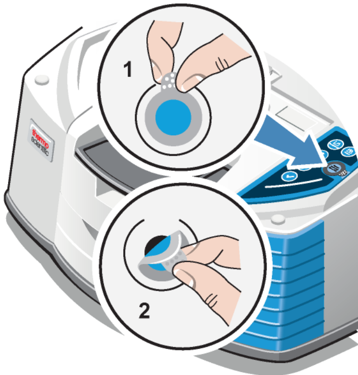
Figure 1-1: Removing the old humidity indicator
