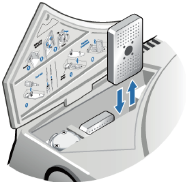
Figure 1-3: Lifting the desiccant cover
