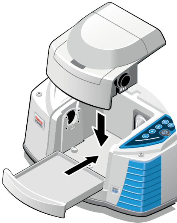
Figure 1-1: Install transmission accessory
