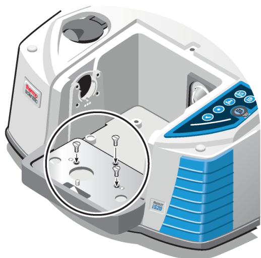
Figure 1-2: Sample compartment extension kit screw installation
