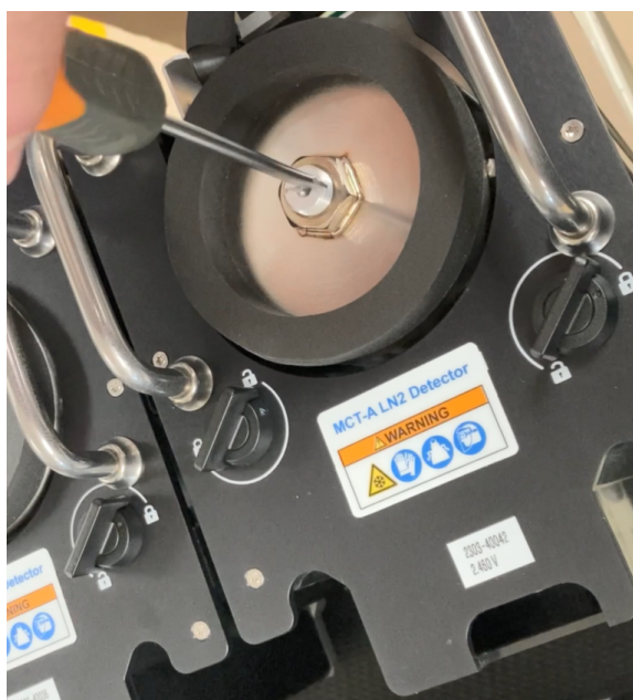
Figure 4-1: Reinstalling the larger restraint
