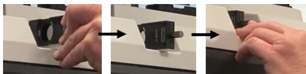
Figure 3-2: Insert Wollaston prism into base slot
