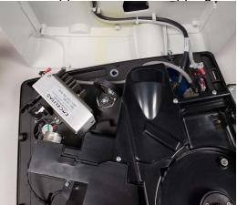
3. Using Phillips screw driver remove two screws holding the 9 pin connector.
