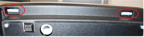
A. Lift off top cover, rotating backwards, being careful not to overstress the Printer and Display cables. Place cover side under the base of instrument to support cover from tipping.
