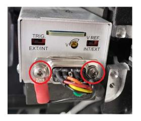
4. Using Phillips screw driver remove two screws holding the machined bracket to casting.
