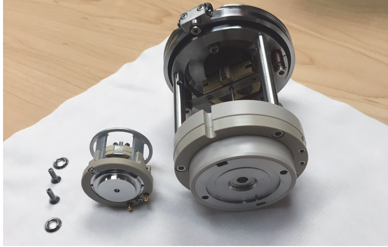
Figure 90. MP00 assembly removed from the cage (TSQ Fortis and TSQ Fortis Plus)
