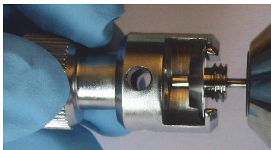
Figure 80. Pulling the tube out of the spray cone
