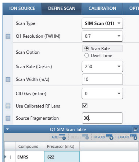
Figure 56. Scan parameters for a TSQ Series II MS (except for a TSQ Fortis model) in positive mode
