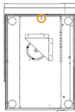
Mechanical Emergency Door Release on the downside
