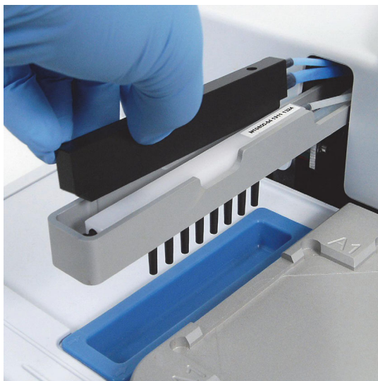
Figure 2–13. Fitting the blank wash head onto the left position of the wash head arm
