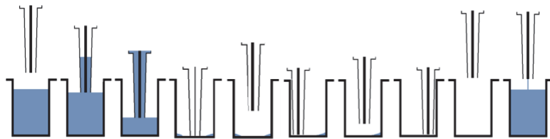
Figure 1-5. Principle of washing step (Sweep3)
