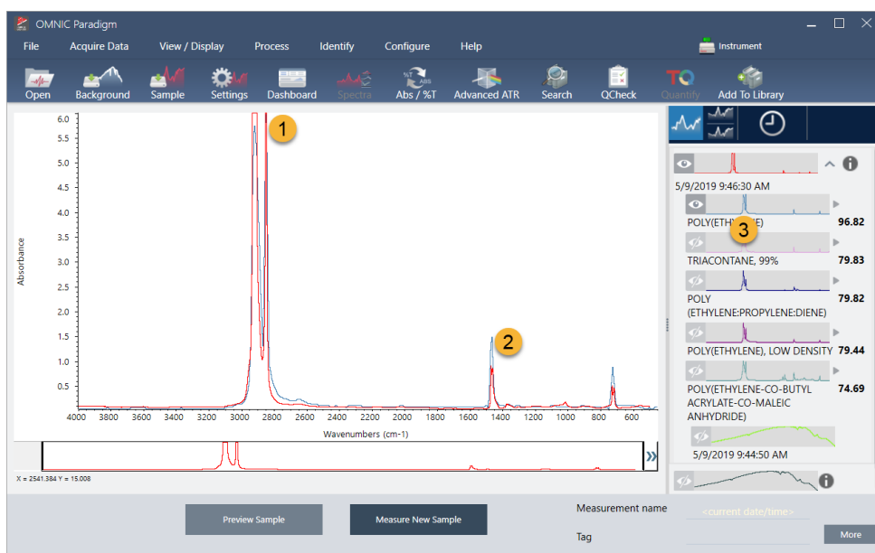
Figure 3-4: Sample and top search result displayed together using the same Y-axis scale
