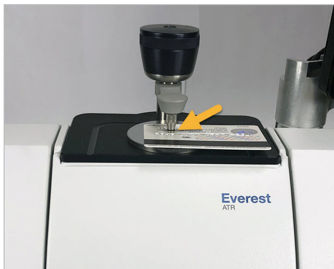
Figure 3-2: Measure a solid with ATR
