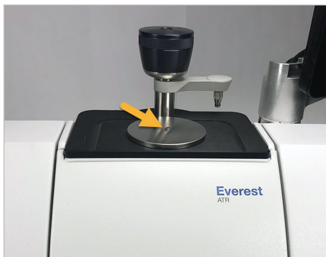
Figure 3-1: Measure a liquid with ATR
