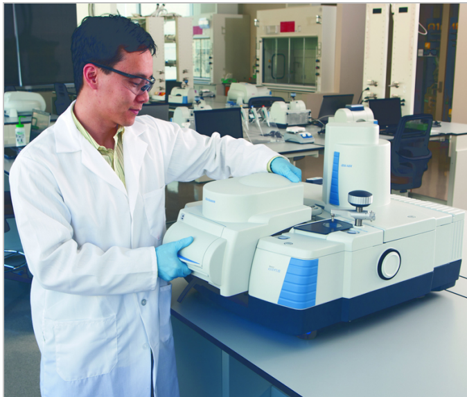
Figure 1-4: Installing the Raman Module
