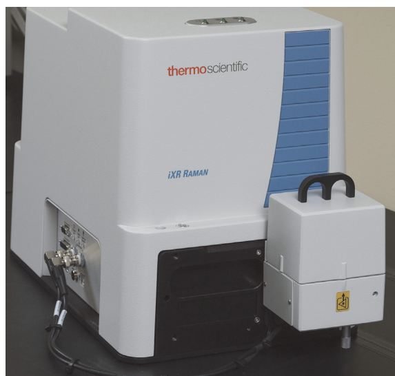
Figure 10. The macro sampling accessory shown installed and with the top cover on
