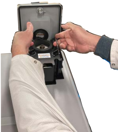
Figure 3-11: Lifting / inserting a detector
