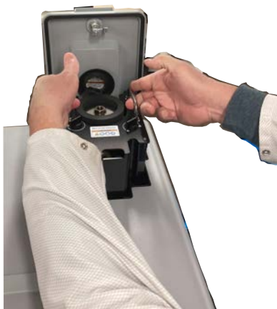
Figure 3-4: Lifting / inserting a detector
