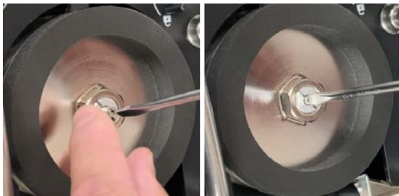
Figure 4-2: Reinstalling the smaller restraint
