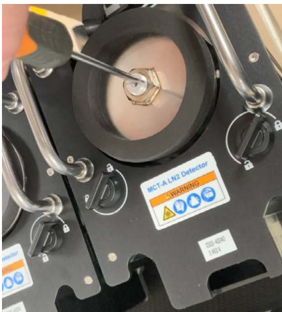
Figure 4-1: Reinstalling the larger restraint
