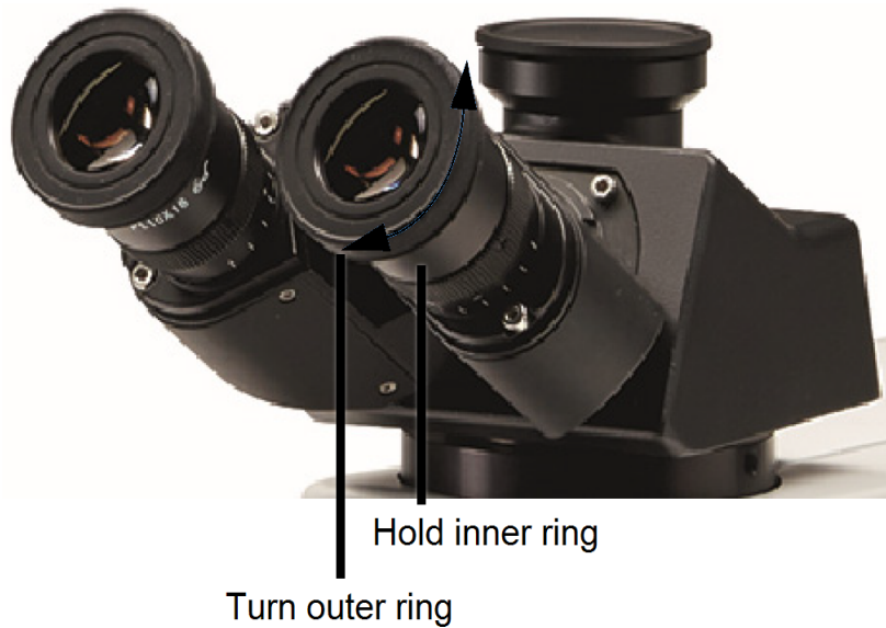
Figure 3-5: Focusing the eyepiece reticle
