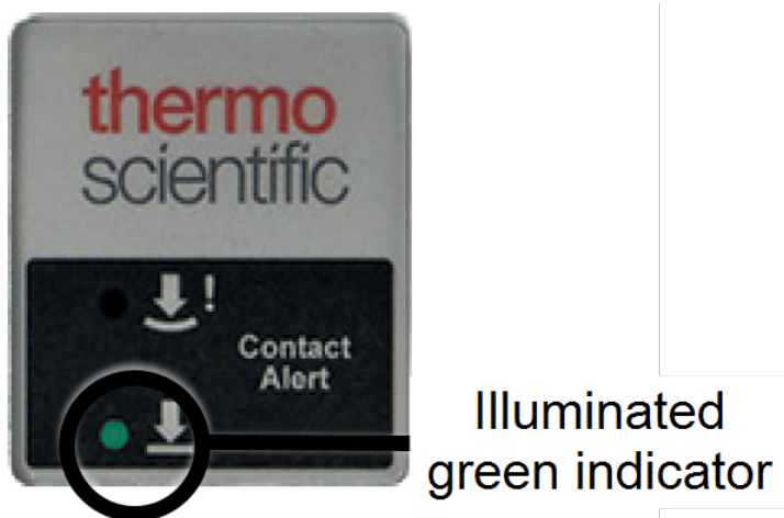
Figure 4-18: Sample spectrum in contact with the ATR crystal
