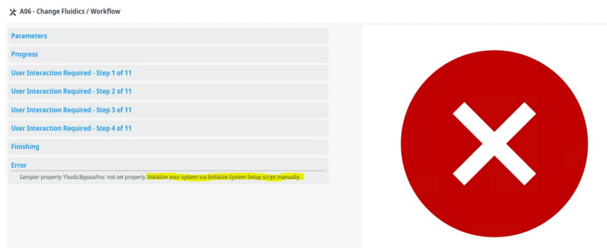
Figure 54: Error message caused by incomplete execution of script A06 – change fluidics / workflow
