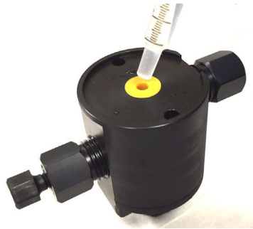
Figure 9. Filling the head cavity with deionized water (plastic syringe shown)
