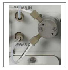
the eluent reservoir. The valve opens automatically when the pump is started and closes when the pump is turned off. The valve can also be opened and closed manually from the Chromeleon Control panel (see Section 2.3.1). This lets you perform service procedures on pump components without eluent leaks occurring.
