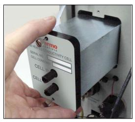
Figure 5-13. Removing the Cell Assembly
