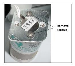
Figure 5-20. Removing the Eluent Valve Mounting Plate
