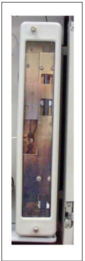
The column heater provides temperature control for the separator and guard column.
