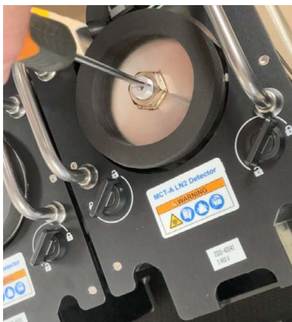
Figure 4-1: Reinstalling the larger restraint
