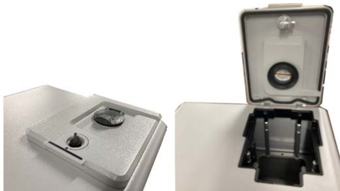
Figure 3-2: Latch: locked position and unlocked position
