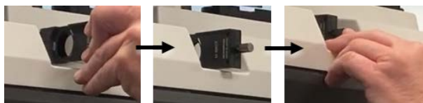
Figure 3-2: Insert Wollaston prism into base slot
