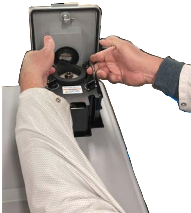
Figure 3-11: Lifting / inserting a detector
