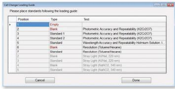
Verification tests specific to USP 2015 can be automatically selected to be used with or without a mercury lamp
