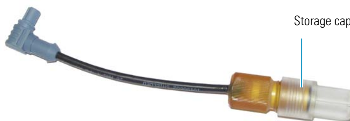
Figure 25. pH-Ag/AgCl reference electrode in storage cap
