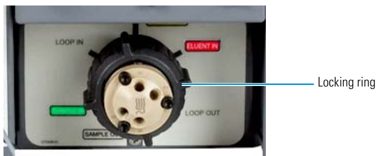
Figure 78. High-pressure valve locking ring
