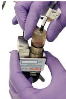
Figure 104. Installation of the pH-Ag/AgCl reference electrode in the reference electrode well
