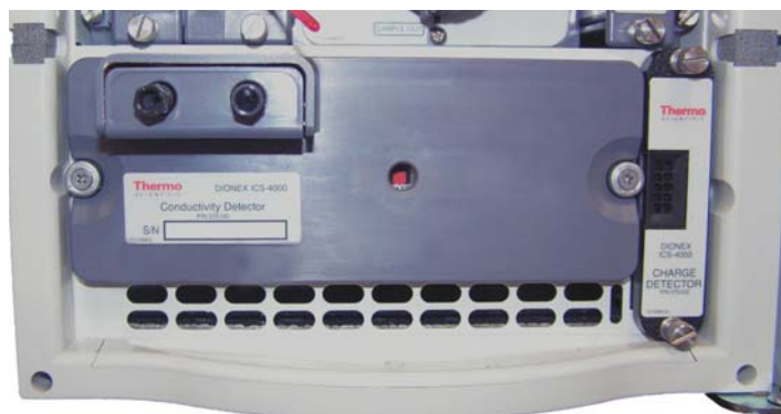
Figure 92. QD installed in chromatography compartment
