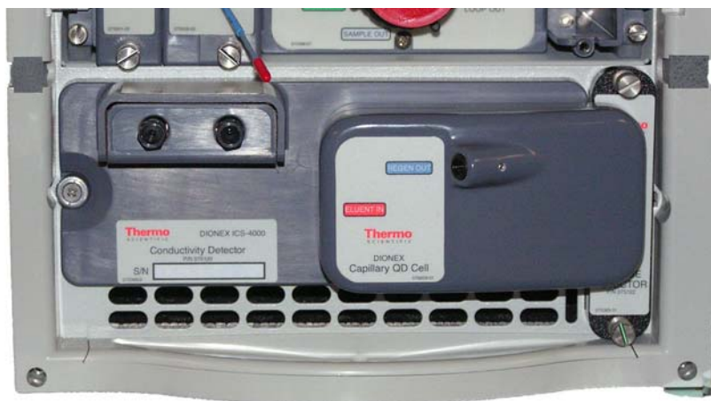
Figure 91. Dionex QDC 300 (Capillary) installed on Dionex ICS-4000 Conductivity Detector
