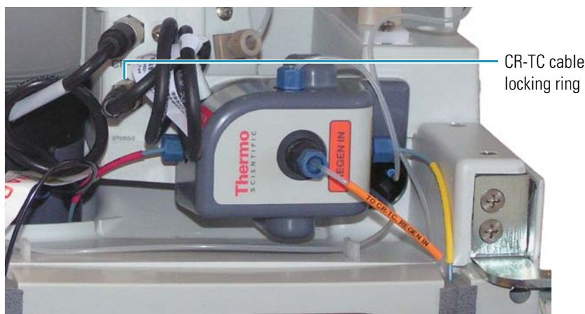
Figure 76. CR-TC electrical cable
