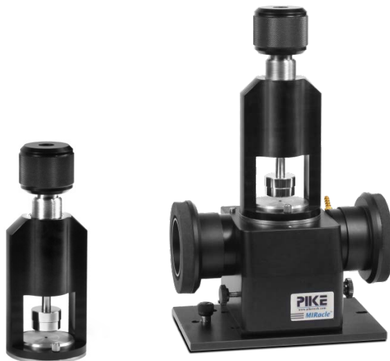
Figure 10: The high pressure, Sealed Sample Chamber Clamp for the MIRacle Single Reflection ATR accessory allows the clamp/crystal plate assembly to be removed from the MIRacle base mounted in the spectrometer to a protective environment for sample loading and handling. Typical applications include studies of toxic or chemically aggressive solids and powders. Dedicated Sealed Sample Chamber Clamp crystal plates, available in diamond, ZnSe or Ge, must be ordered separately.
