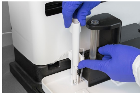
FIGURE 2-12 Installing the Rinse Station
