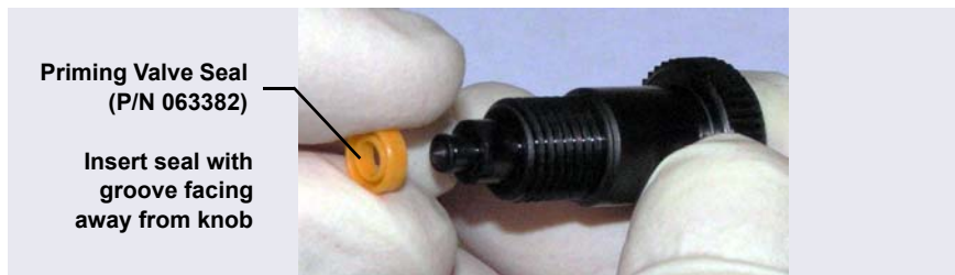
Figure 9-12. Replacing the Priming Valve Seal
