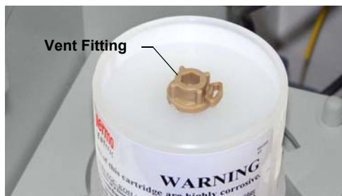
Figure 9-15. Capillary Dionex EGC Vent Fitting
