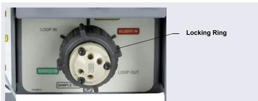
Figure 9-36. Unscrew the Locking Ring (Valve in IC Cube Shown)
