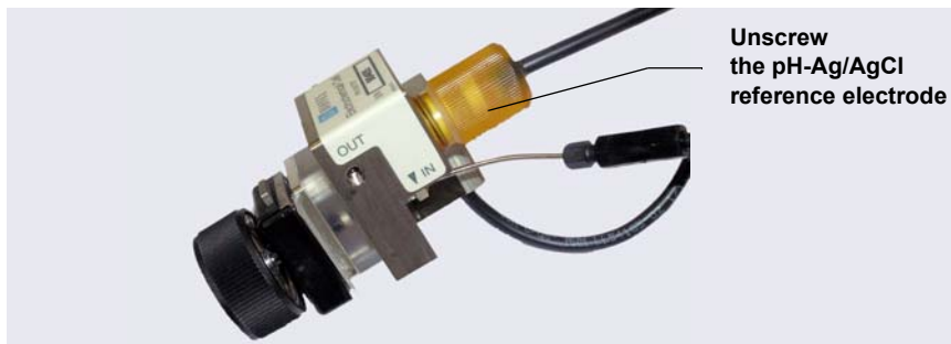
Figure 9-57. Removing the pH-Ag/AgCl Reference Electrode (Cell Configured for Analytical IC Shown)
