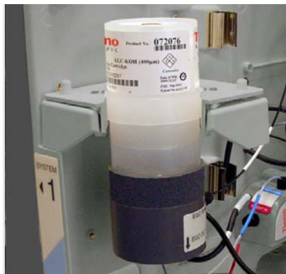
Figure 9-20. Capillary Dionex EGC Installed on Holder
