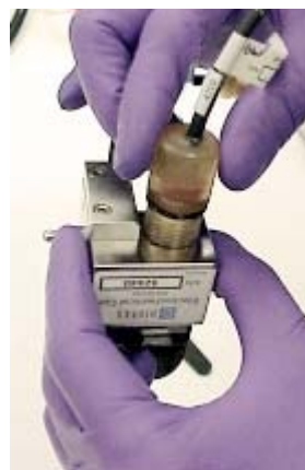
Figure 9-63. Installing the pH-Ag/AgCl Reference Electrode In the Reference Electrode Well
