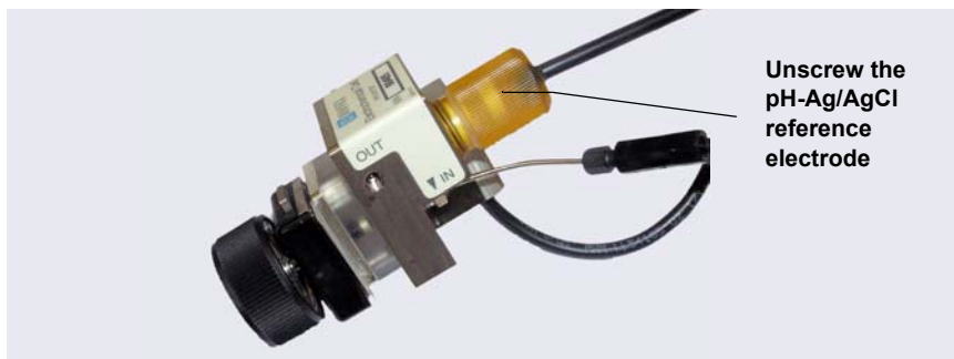
Figure 9-65. Removing the pH-Ag/AgCl Reference Electrode (Cell Configured for Analytical IC Shown)
