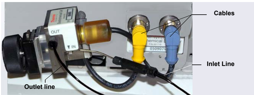
Figure 9-53. Disconnecting the ED Cell (Cell configured for analytical IC shown)
