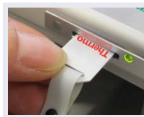
Figure 9-75. Inserting a Column ID Chip Card
