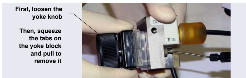
Figure 9-54. Disassembling the ED Cell (Cell Configured for Analytical IC Shown)
