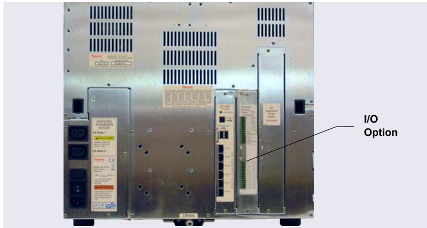
Figure 9-39. DC Rear Panel: I/O Option Installed
