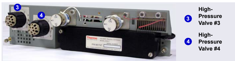
Figure 8-7. High-Pressure Valves #3 and #4 (On AM)
