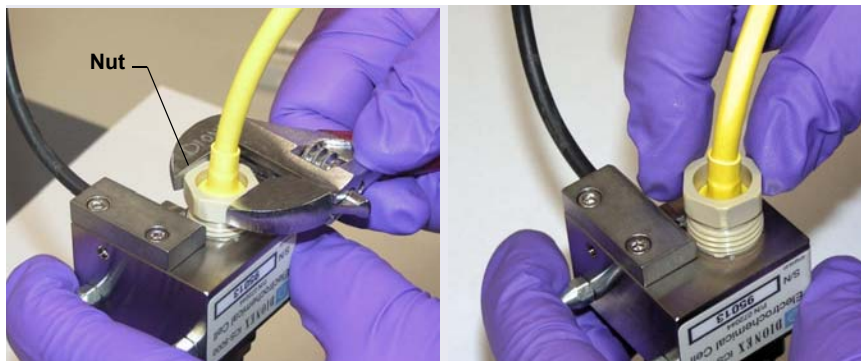
Figure 9-67. Unscrewing the PdH Reference Electrode Nut
