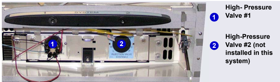
Figure 8-5. High-Pressure Valves #1 and #2 (In DC Lower Compartment)
