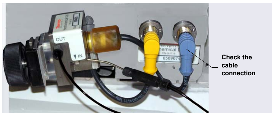
Figure 8-8. ED Cell Electrical Connections
