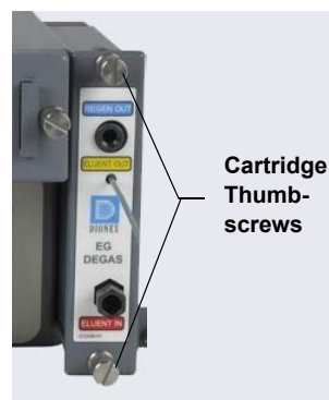
Figure 9-41. Capillary Cartridge Thumbscrews (EG Degas Cartridge Shown)
