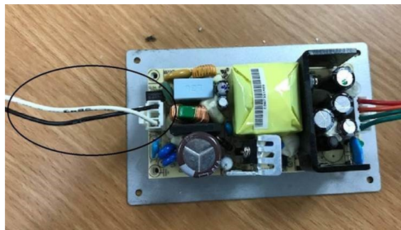
Figure 4. Discard AC connector
