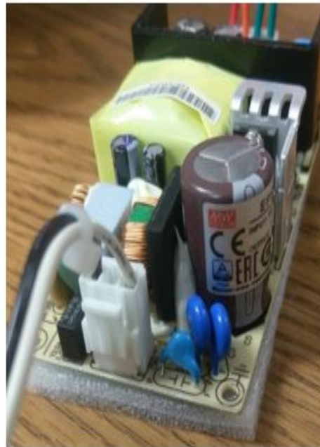
Figure 6. Power supply AC connection
