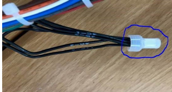
Figure 5. Connect black to black using 370398
