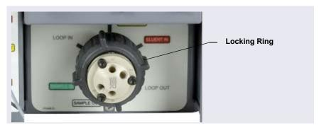
Figure 9-35. Unscrew the Locking Ring (Valve in IC Cube Shown)
