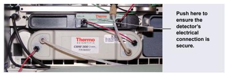
Figure 8-3. Conductivity Detector Connection
