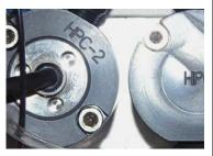
A Capillary Pump High-Pressure Upgrade Kit (P/N 075994) is available for converting a lower pressure rated capillary IC pump to a higher pressure rated pump. The kit includes the HPC-2 secondary pump head and high-pressure pump seals.
