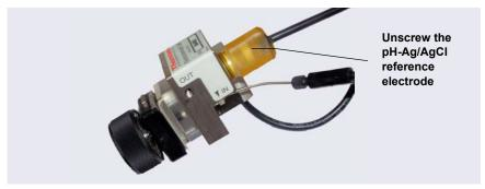
**Figure 9-64.** Removing the pH-Ag/AgCl Reference Electrode (Cell Configured for Analytical IC Shown)
