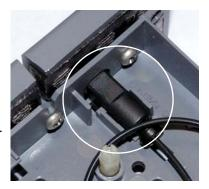
Figure 9-44. Separator Column Outlet Fitting
