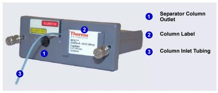
Figure 9-48. Column Cartridge Closed
