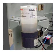
Figure 9-20. Capillary EGC Installed on Holder
