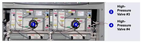
**Figure 8-6.** High-Pressure Valves #3 and #4 (On IC Cubes)
