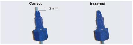
**Figure 9-1.** Correct and Incorrect Ferrule and Fitting Bolt Placement for Capillary Tubing Connections (High-Pressure Fitting and Ferrule Shown)
