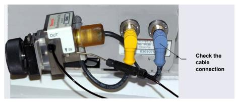
Figure 8-8. ED Cell Electrical Connections
