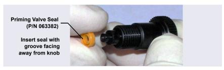
Figure 9-12. Replacing the Priming Valve Seal
