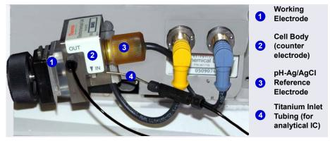
**Figure 2-30.** ED Cell with pH-Ag/AgCl Reference Electrode (Cell Configured for Analytical IC Shown)
