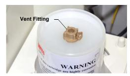
Figure 9-15. Capillary EGC Vent Fitting
