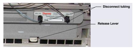
Figure 9-51. Disconnecting the CD Liquid Lines (Capillary CD shown)
