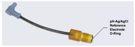
Figure 9-65. Removing the pH-Ag/AgCl Reference Electrode O-Ring
