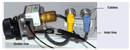
**Figure 9-52.** Disconnecting the ED Cell (Cell Configured for Analytical IC Shown)
