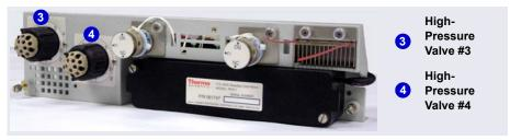
Figure 8-7. High-Pressure Valves #3 and #4 (On AM)
