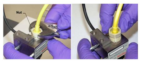
Figure 9-66. Unscrewing the PdH Reference Electrode Nut
