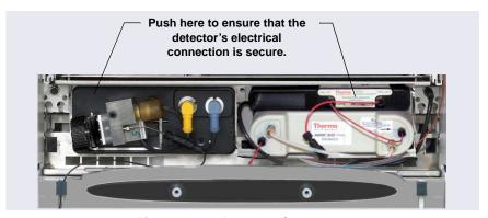
Figure 8-1. Detector Connection
