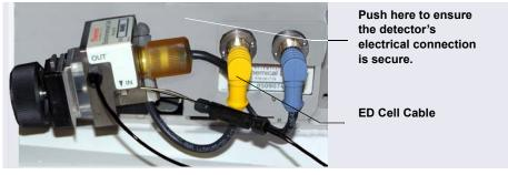
Figure 8-4. Electrochemical Detector Connection (Analytical Cell Shown)
