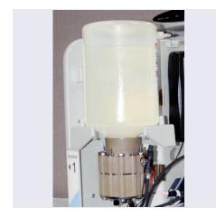
Figure 9-24. Analytical EGC Installed on Holder
