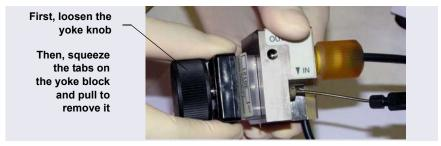
**Figure 9-53.** Disassembling the ED Cell (Cell Configured for Analytical IC Shown)
