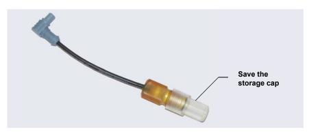
Figure 9-57. pH-Ag/AgCl Reference Electrode in Storage Cap
