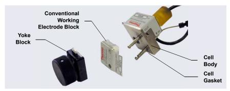
Figure 9-54. ED Cell Components
