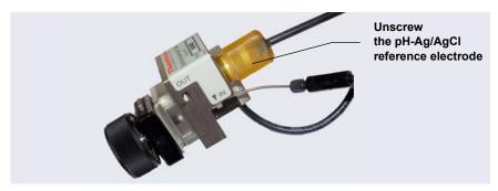
**Figure 9-56.** Removing the pH-Ag/AgCl Reference Electrode (Cell Configured for Analytical IC Shown)
