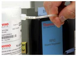
Figure 9-16. Analytical EGC Vent Line
