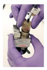
**Figure 9-62.** Installing the pH-Ag/AgCl Reference Electrode In the Reference Electrode Well
