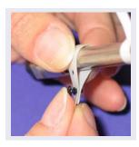
Figure 9-73. Attaching the Column ID System to the Column
