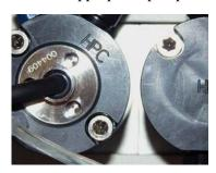
• **HPC-2** is stamped on the secondary pump heads of the newer (higher pressure rated) capillary IC pumps.
