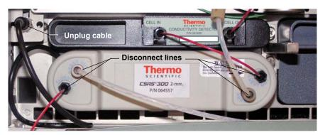
Figure 9-50. Disconnecting the Suppressor Liquid Lines and Cable
