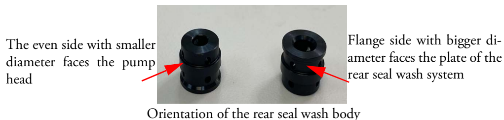
Figure 67. Rear seal wash body
