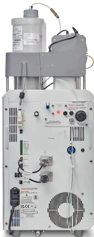
Figure 22. Dionex Inuvion IC System rear panel
