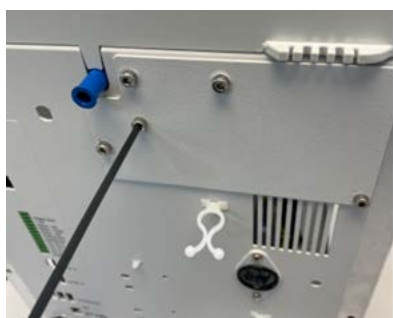
Figure 90. Digital pressure regulator port location (with port cover)
