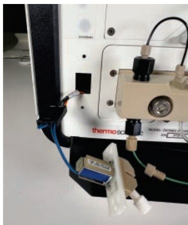
Figure 75. Eluent valve control wires
