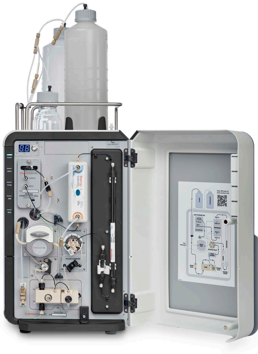
Figure 5. Dionex Inuvion Core IC System component panel (with column holder and regenerant pump installed)
