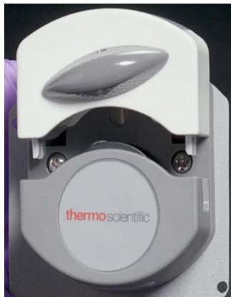
Figure 32. Tubing placed between the rollers of the regenerant pump
