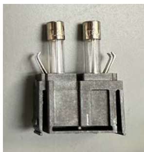
Figure 97. Main power fuse holder
