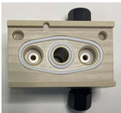
Figure 66. View of piston seal and support ring in the analytical pump head
