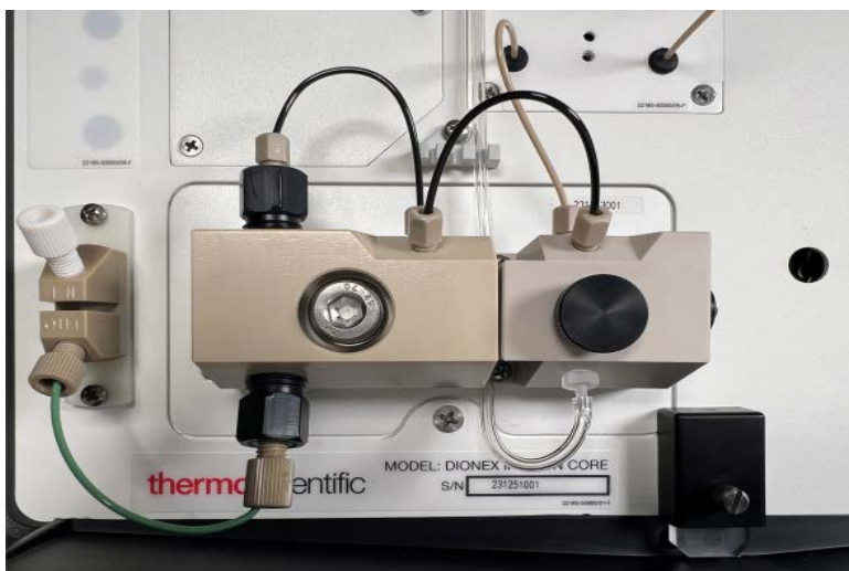
Figure 16. Dionex Inuvion IC System analytical pump assembly (pump to the left, pressure transducer to the right)
