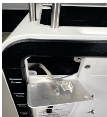
Figure 87. Digital display back cable
