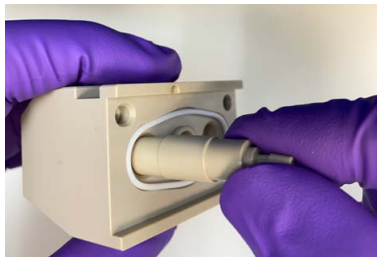
Figure 65. Inserting the piston seal with the piston seal tool
