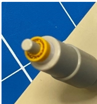
Figure 64. Piston seal and support ring placed on the seal tool (spring side up)
