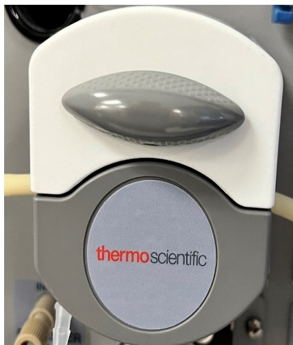
Figure 38. Closing the regenerant pump cover after tubing installation
