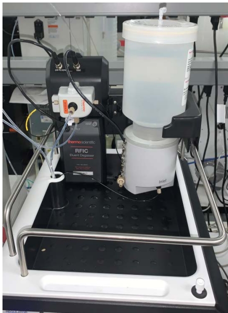
Figure 13. Dionex Inuvion IC System eluent organizer area (with Dionex EGC, Dionex CR-TC, and RFIC eluent degasser installed)
