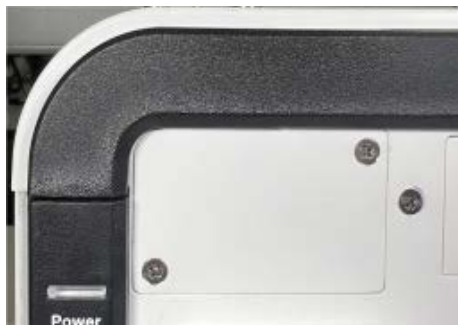
Figure 86. Blank cover without digital pressure regulator display
