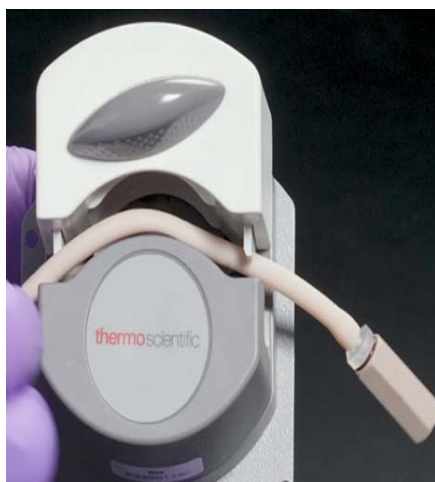
Figure 32. Tubing placed between the rollers of the regenerant pump
