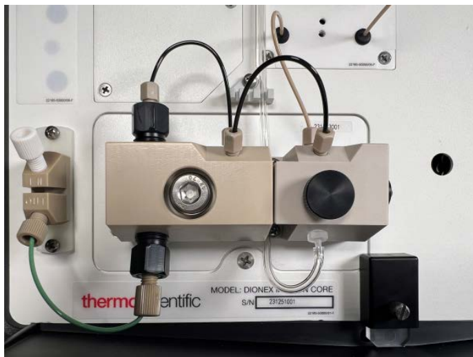
Figure 49. Analytical pump head fluidic connections
