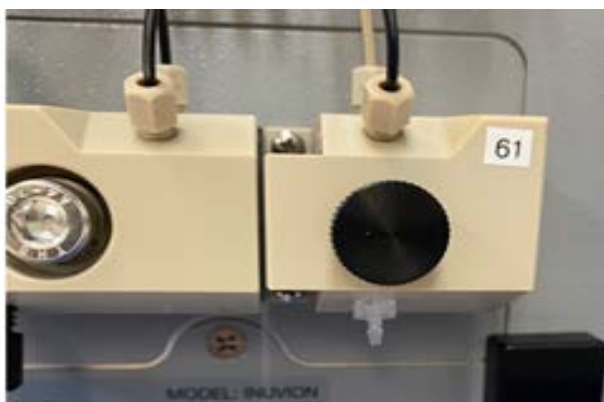
Figure 17. Dionex Inuvion IC System pressure transducer (marked with “61”)
