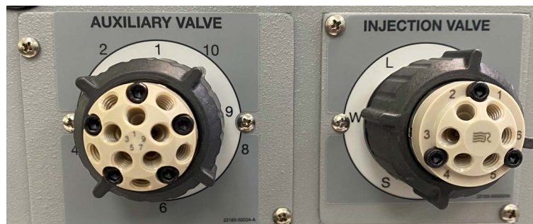
Figure 35. Auxiliary and injection valve black locking rings
