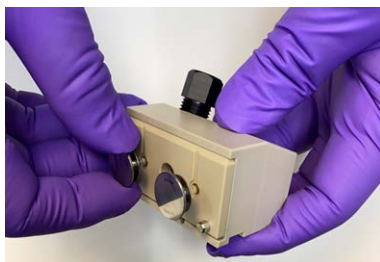
Figure 55. Removing the piston from analytical pump
