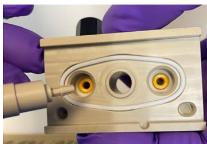
Figure 61. Removing an analytical pump seal with the seal tool
