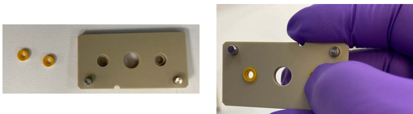
Figure 71. Installing the rear seals
