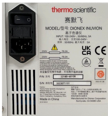
Figure 96. Main power switch and fuse holder
