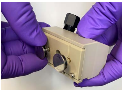
Figure 73. Reinstalling the pistons into the analytical pump head assembly
