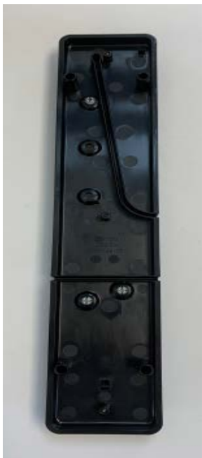
Figure 12. Injection port plumbing channel through the column heater cover
