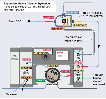
*Figure 10-47.* Flow Schematic for Hydrating the Suppressor Eluent Chamber in a Capillary IC System
