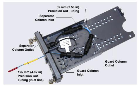
*Figure 10-54.* 150 mm Separator Column and 35 mm Guard Column Installed in Capillary Column Tray
