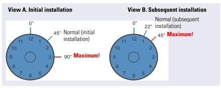
Figure 10-2. IC PEEK Viper Fitting Installation
