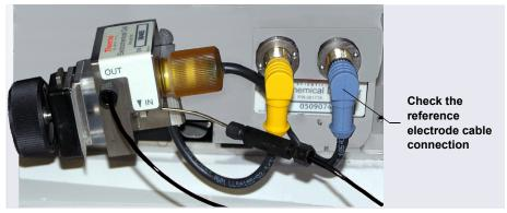
Figure 9-8. ED Cell Electrical Connections
