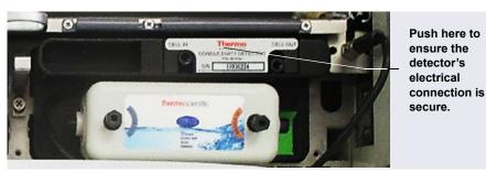
Figure 9-3. Conductivity Detector Connection
