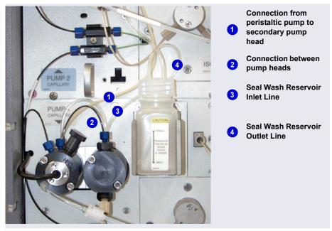
Figure 4-3. Piston Seal Wash Connections to Pump 1
