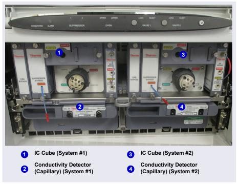
Figure 2-18 shows the upper compartments of a DC that is configured for two capillary IC systems. Both systems are configured for conductivity detection.
