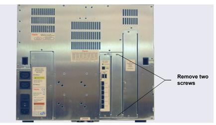
Figure 10-39. DC Rear Panel: Removing the I/O Option Cover Plate
