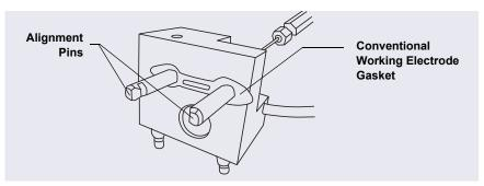
Figure 10-62. ED Cell Gasket for Conventional Working Electrodes
