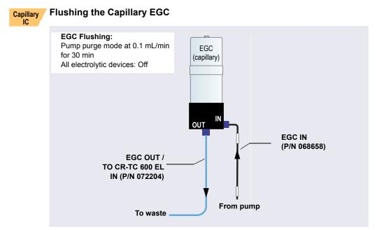
Figure 10-21. Flow Schematic for Flushing the Dionex EGC (Capillary)
