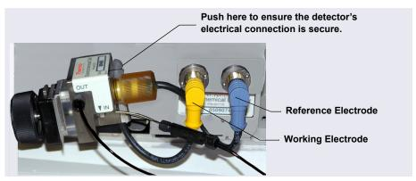
electronics connector on the back of the detector is securely connected to the receptacle on the detector compartment.
