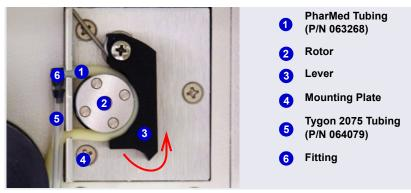
Figure 10-10. Peristaltic Pump for Seal Wash System
