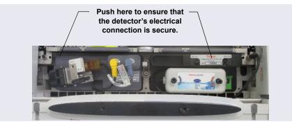
Figure 9-1. Detector Connection
