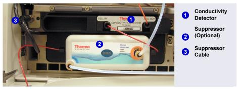
Figure 2-28. Analytical Conductivity Detector with Suppressor (System #1)
