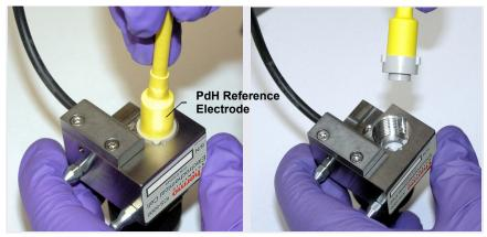
*Figure 10-72.* Removing the PdH Reference Electrode from the Reference Electrode Well
