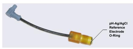
Figure 10-70. Removing the pH-Ag/AgCl Reference Electrode O-Ring
