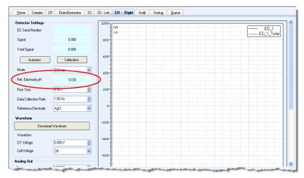
Figure 4-1. Monitoring the pH-Ag/AgCl Reference Electrode pH
