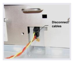
Figure 10-36. Leak Sensor Cable
