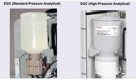
Figure 10-26. Analytical Dionex EGC Installed in Holder
