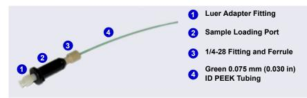
Figure 10-34. Sample Loading Port Connection
