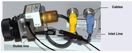
*Figure 10-59.* Disconnecting the ED Cell (Cell Configured for Analytical IC Shown)
