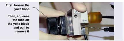
**Figure 10-60.** Disassembling the ED Cell (Cell Configured for Analytical IC Shown)
