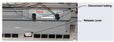
Figure 10-58. Disconnecting the CD Liquid Lines (Capillary CD Shown)
