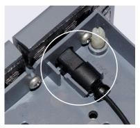
Figure 10-49. Separator Column Outlet Fitting
