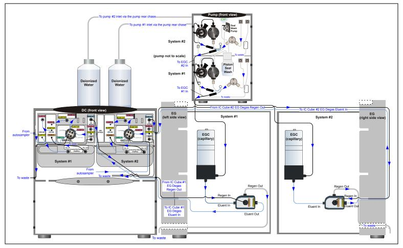
Figure 3-1. Capillary IC: Dual RFIC-EG System (CD/CD)
