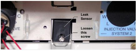
Figure 10-35. Leak Sensor
