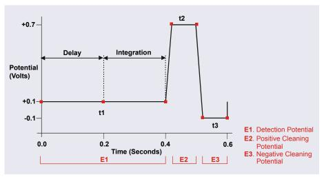
Figure 2-46. Example Pulsed Amperometry Waveform
