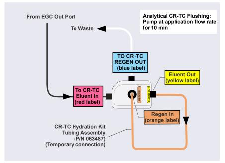
Figure 10-30. Plumbing for Hydrating an Analytical Dionex CR-TC 600
