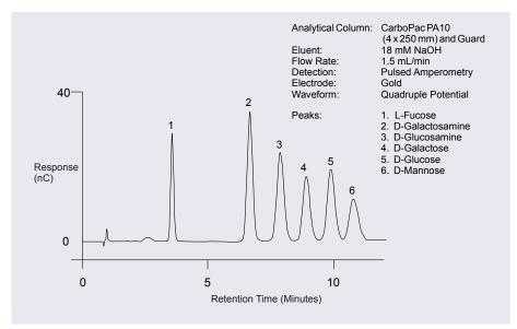
Figure 2-49. Example Chromatogram for a Pulsed Amperometry Application
