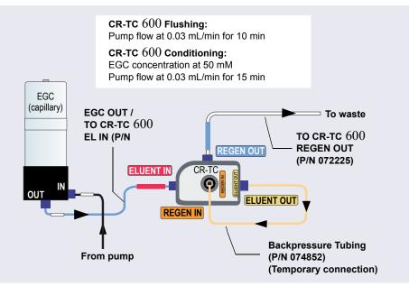
*Figure 10-28.* Flow Schematic for Flushing and Conditioning the Dionex CR-TC 600 (Capillary)
