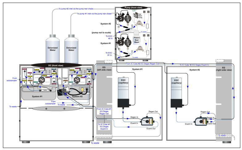
Figure 3-2. Capillary IC: Dual RFIC-EG System (CD/ED)
