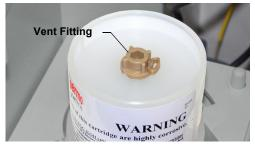
Figure 10-16. Capillary Dionex EGC Vent Fitting
