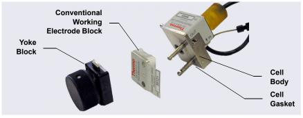
4. Carefully separate the parts (see <u>Figure 10-61</u>).
