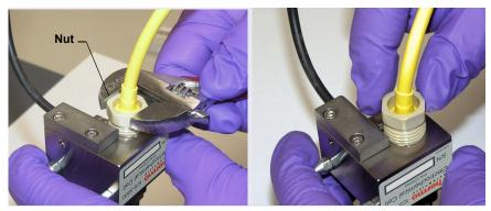
Figure 10-71. Unscrewing the PdH Reference Electrode Nut
