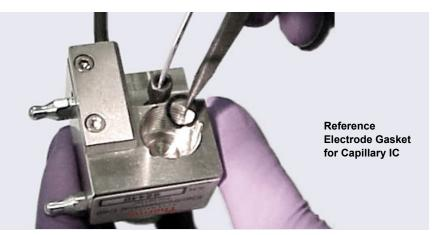
Figure 10-65. Reference Electrode Gasket for Capillary IC
