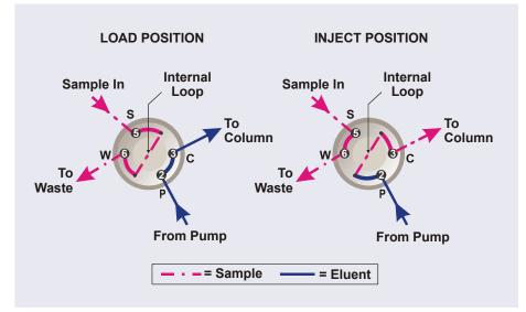
Figure 2-25 shows flow schematics for the 4-port valve.
