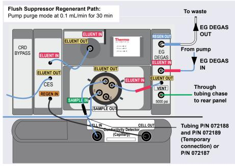
3. Connect the pump to the regenerant path as shown in Figure 10-46.
