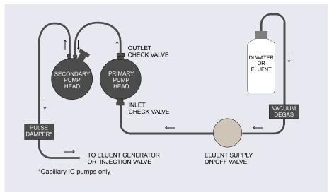
Figure 2-5. Isocratic Pump Flow Schematic
