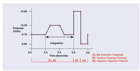
Figure 2-47. Example Integrated Amperometry Waveform
