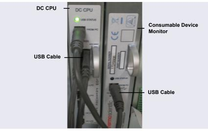
Figure 10-43. Dionex Consumable Device Monitor Connected to CPU Board
