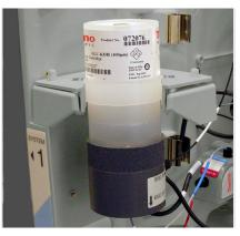
Figure 10-20. Capillary Dionex EGC Installed on Holder
