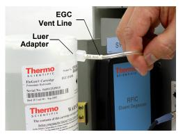
Figure 10-17. Analytical Dionex EGC Vent Line (Standard-Pressure Cartridge Shown)
