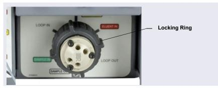
Figure 10-37. Unscrew the Locking Ring (Valve in IC Cube Shown)
