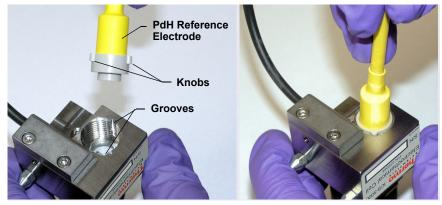
*Figure 10-75.* Inserting the PdH Reference Electrode Fitting into the Reference Electrode Well
