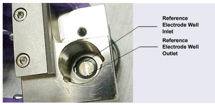
*Figure 10-66.* Reference Electrode Well with Reference Electrode Gasket for Capillary IC Installed
