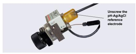
*Figure 10-69.* Removing the pH-Ag/AgCl Reference Electrode (Cell Configured for Analytical IC Shown)
