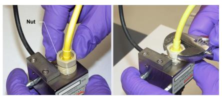
Figure 10-76. Installing the PdH Reference Electrode Nut
