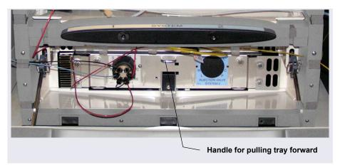
Figure 2-23. DC Lower Compartment Tray Handle
