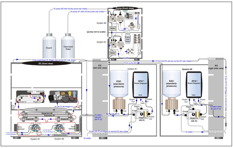
Figure 3-7. Analytical IC: Dual RFIC-EG System (CD/ED)
