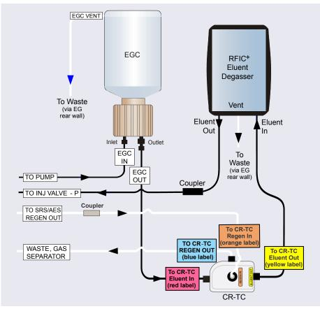
the appropriate figure when performing Dionex EGC and Dionex CR-TC 600 service procedures for an analytical IC system.
