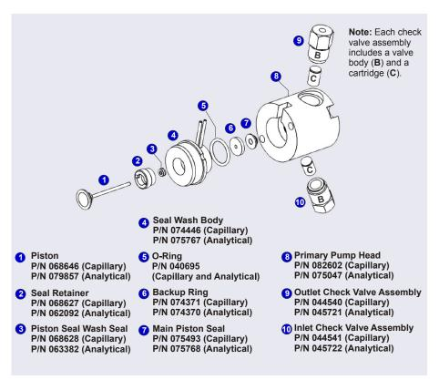
Figure 10-7. DP/SP Pump: Primary Pump Head Assembly
