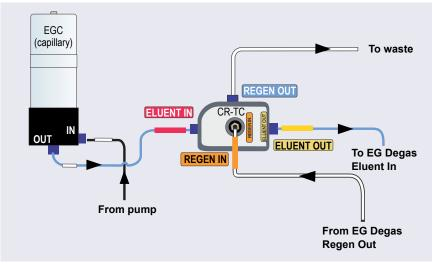
Figure 10-29. Capillary Dionex CR-TC 600 Plumbing Diagram: Installation Completed
