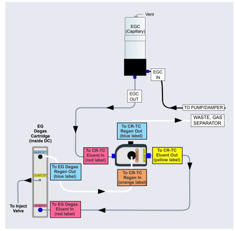
Figure 2-13. EG Flow Schematic Example for Capillary IC
