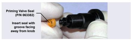
Figure 10-13. Replacing the Priming Valve Seal
