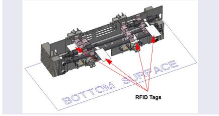
In <u>Figure 5-5</u>, RFID tags are parallel to the floor of the DC, and point to both the front and back of the module.
