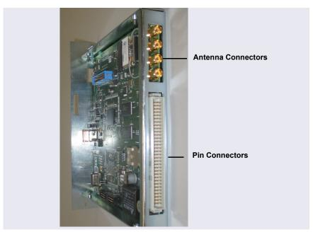
antenna connectors are on top and the pin connectors are below (see Figure 10-42).
