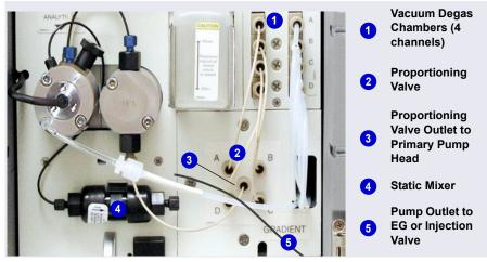
Figure 2-4. Analytical Gradient Pump Components
