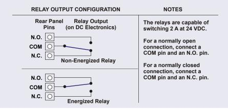
Figure 2-36. Relay Output Configuration
