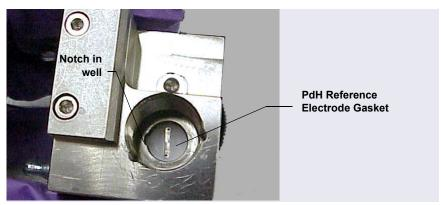
Figure 10-73. Removing the PdH Reference Electrode Gasket
