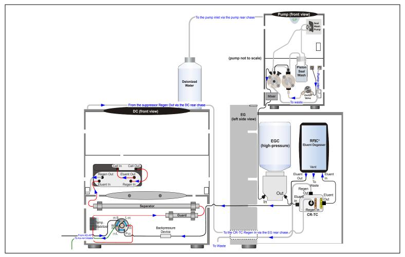
Figure 3-5. Analytical IC: Single RFIC-EG System (CD)
