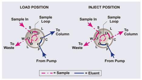
Figure 2-26. Injection Valve Flow Schematics (6-Port Valve)
