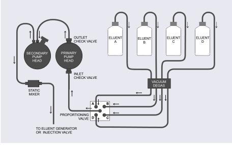
Figure 2-6. Gradient Pump Flow Schematic
