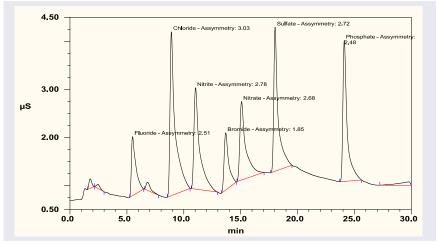
Figure 9-2. Tailing Peaks Caused by Incorrectly Installed Capillary Tubing Fittings
