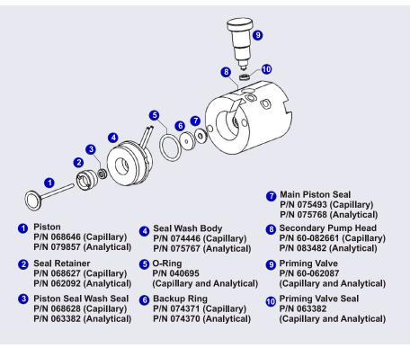
Figure 10-8. DP/SP: Secondary Pump Head Assembly
