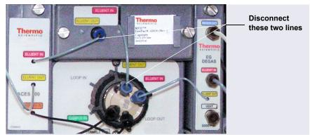
*Figure 10-48.* Disconnect Capillary Tray Eluent Lines (Conductivity System Plumbing Shown)
