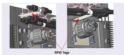
Figure 5-6. RFID Tags Attached to Underside of Columns
