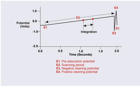
Figure 2-48. Example Scanning Waveform
