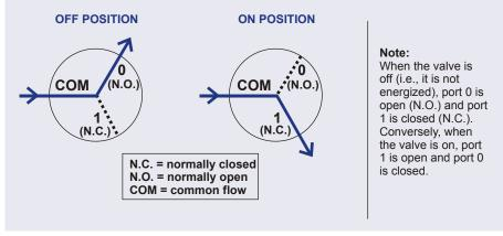
Figure 2-43. Three-Way Low-Pressure Valve Flow Schematics
