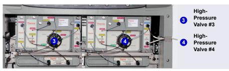
Figure 9-6. High-Pressure Valves #3 and #4 (in IC Cubes)
