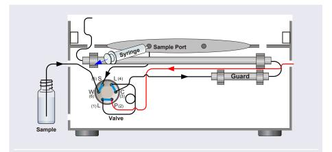
Figure 5-2. Loading Sample with a Vacuum Syringe (Pull Method)
