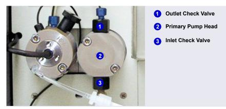
7. The check valves are installed in the primary pump head (see Figure 10-4).
