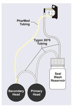
Figure 10-11. Piston Seal Wash Tubing Connections
