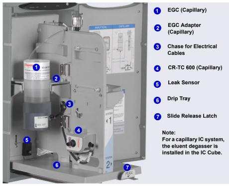
To access components for maintenance or service procedures, push down on the slide release latch and pull the tray forward until it reaches the stop.
