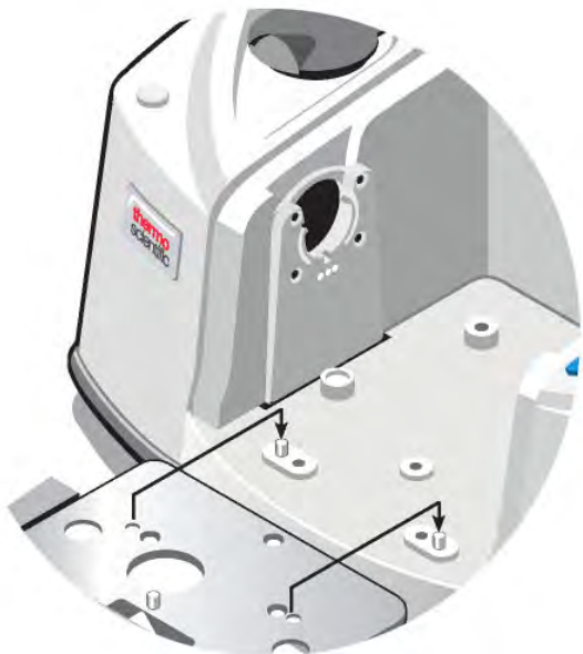
Figure 4-1: Sample compartment extension kit pins
