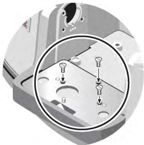
Figure 4-2: Sample compartment extension kit screw installation
