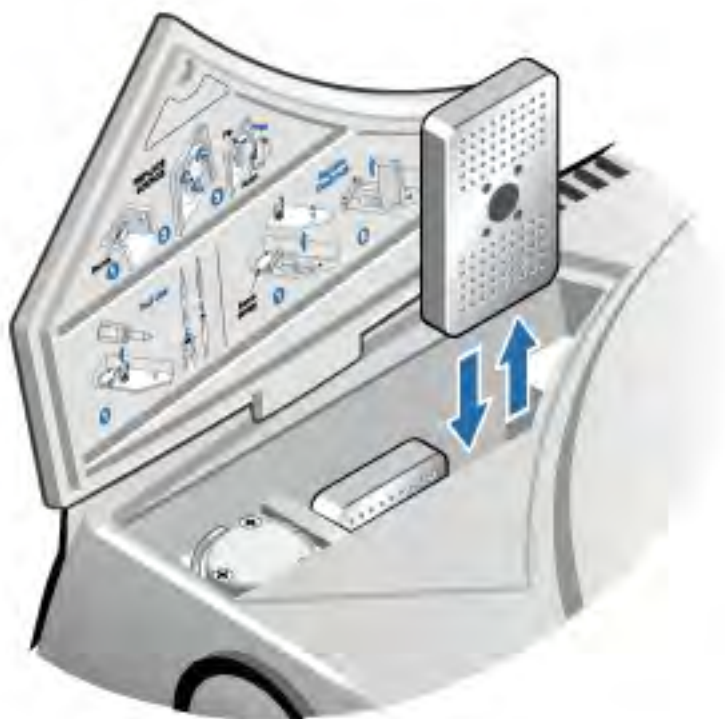
Figure 5-3: Lifting the desiccant cover
