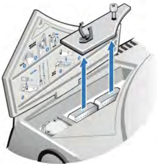
Figure 5-2: Removing desiccant cover.
