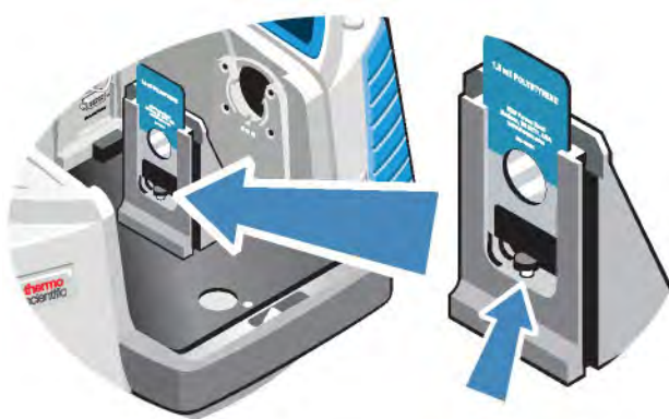
Figure 4-2: Adjust sample height
