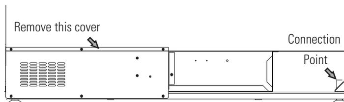
**Figure 1-16.** Cover Plate on Back of Unit
