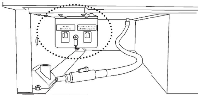
**Figure 1-27.** Location of RS-232 and Remote Alarm Connectors
