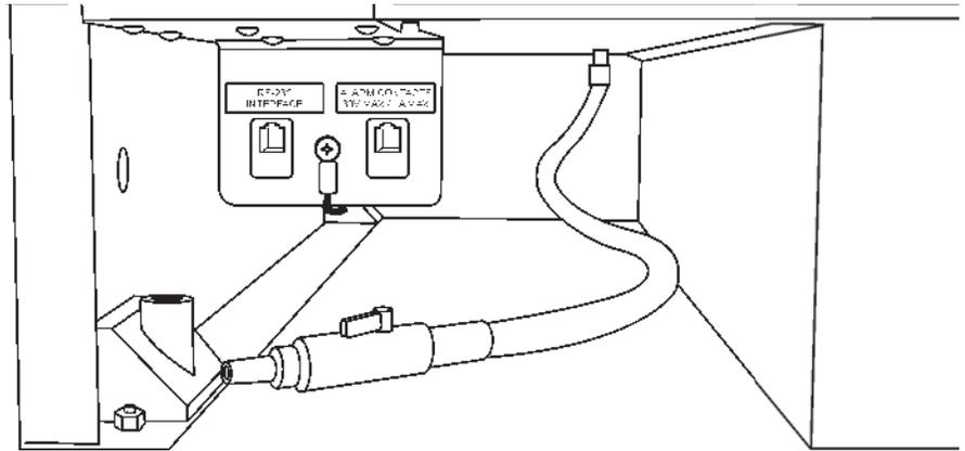
**Figure 1-22.** Chamber Drain
