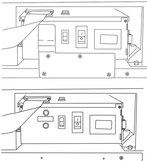
**Figure 4-6.** Relay Enclosure with and without Cover Plate
