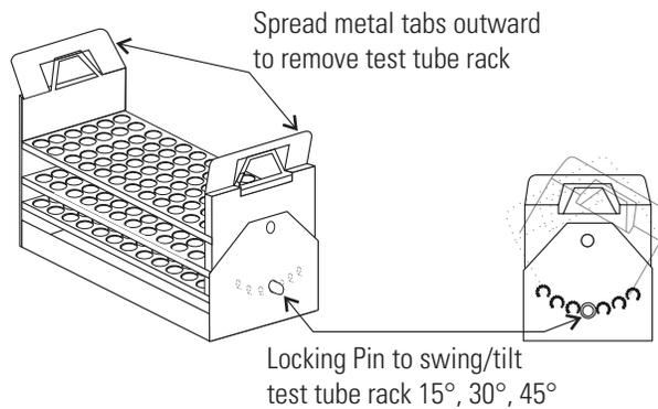
**Figure 1-25.** Test Tube Rack with Swing/Tilt Mechanism
