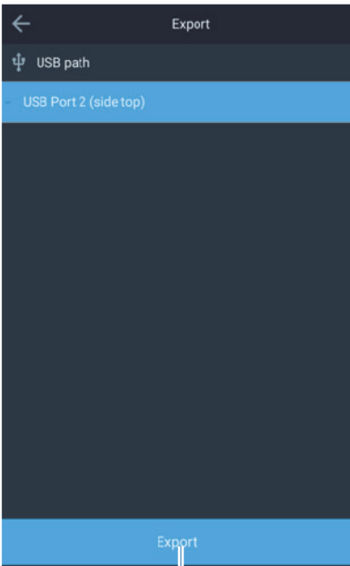
Generate a recovery key onto a USB drive. This key is required during the password reset process and therefore should be kept safely by the administrator.
