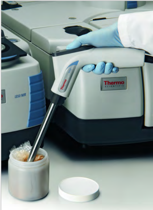
Figure 5-7: Powder sample ready for measurement with a diffuse reflection probe
