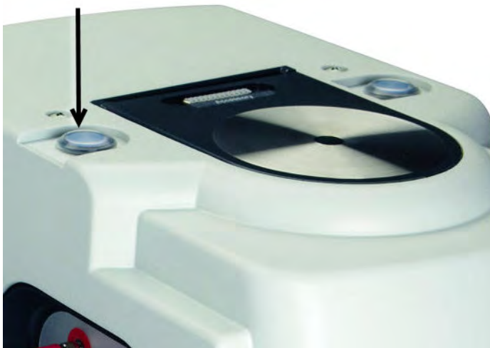
Figure 5-5: Fiber Optic Touch Point
