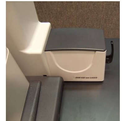
4. System with laser in place and locked.
