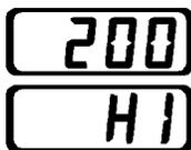
If the actual temperature exceeds the alarm limit, the alarm indicator will light and the Set Display will flash “HI.”
