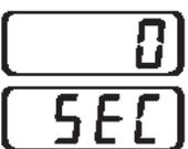
16. The Set Display then shows “SEC” to indicate that the operator must select the number of additional seconds for which the current set temperature will be held. Use the Up or Down Arrow Key to adjust the Actual Display to indicate the desired number of soak seconds (maximum of 59). Press the Menu Key to enter the selected number of soak seconds. Proceed to step 20.
