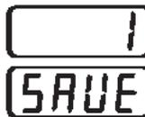
22. *When program editing is complete* the controller will then prompt to save the program, “1 Save”. Press the Menu Key to save the program, or use the Up or Down Arrow Key to change the Actual Display to NO, which will leave the current program as it was found.
