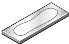
Place the sample upside down on the accessory. A good first sample is a piece of shiny metal, like aluminum, with a thin coating of vegetable oil. Add a drop of oil, and then wipe the metal with a cloth so that a thin layer of oil remains.
