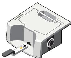
Make sure the slider is pushed in to the second cup (the one closer to the handle). This positions the gold disk in the beam.
