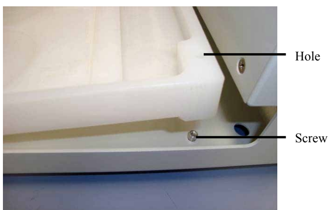
Fig. 31: Installing the universal drip tray
