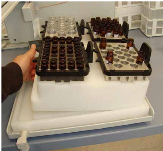
Fig. 11: Removing the rack adapter
