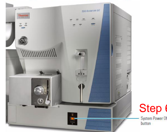
Figure 29. System Power Off button on the front of the electronics module
