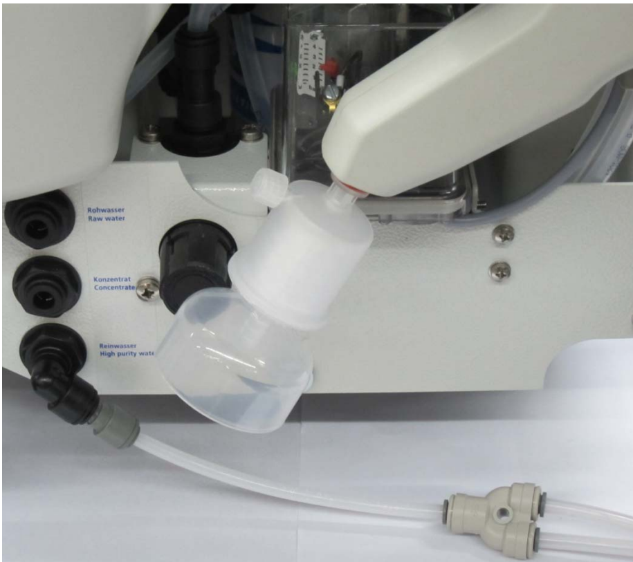
Picture 1 shows accessory dispenser connected to the Pure water supply connection of LabTower RO/TII/EDI/AFT.
